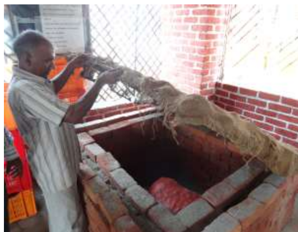
Low cost cold chamber technology of IARI, Pusa adopted at Grameen Hut to keep the vegetable fresh
